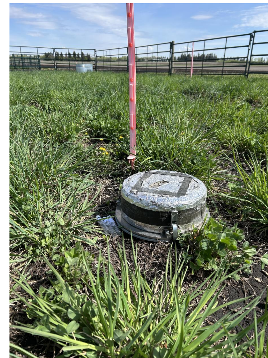
Figure 1. Static gas chamber, with exetainer sampling vials (left)
